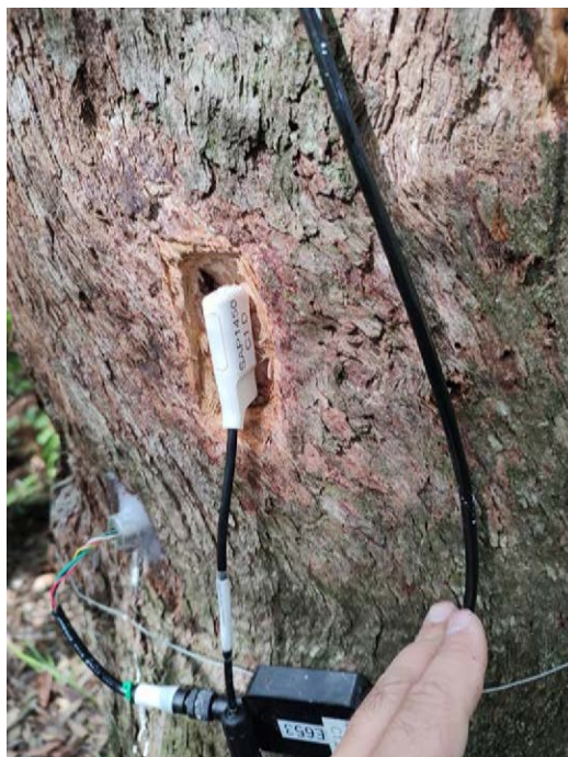
A sensor on tree at the Bullaburra wet sclerophyll site in the Blue Mountains measures tree water stress. Image: Neil Ross, Western Sydney University
