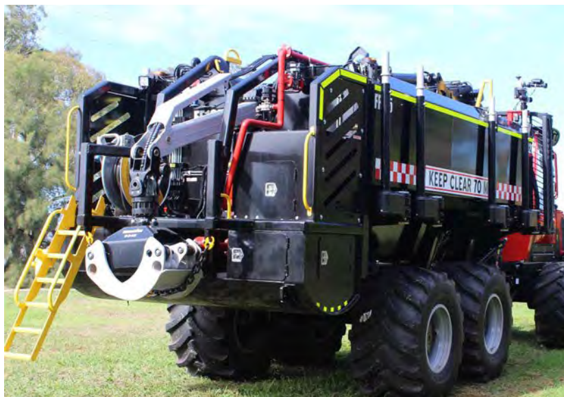
The rear of a Komatsu forwarder fitted with the RL21 Firefighting Kit, showing the robust mounting system, winch and high-visibility safety markings. Image: Komatsu Forest
