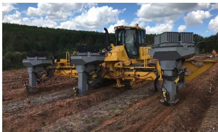
The Komatsu D61EM Planter was one of the mechanised planters discussed by respondents in the report. Image: courtesy Komatsu
