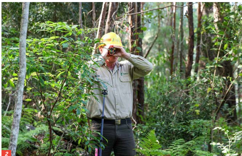
1/ The transponder assists with the capture of digital data. 2/ Rob Lloyd using a Vertex, a precision electronic tool for accurately and instantly measuring tree heights, angles and distances. All images: FCNSW
