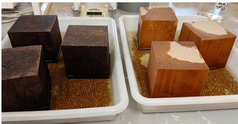
A simple test of water uptake in hyperlignified wood blocks (left) and untreated beech wood blocks (right) shows that the treatment significantly reduces moisture absorption, which helps increase durability. Image: Sune Tjalfe Thomsen
