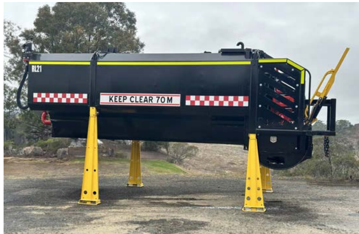
Rodwell's RL21 Kit ready to be mounted on a Komatsu Forwarder.
