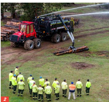
1/ The new Komatsu Fire Forwarder in action in southern NSW, delivering 19,000 litres of high-flow water to rugged pine plantation terrain inaccessible to standard fire tankers.
