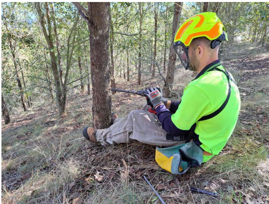
Milwaukee MP18CPD cordless drill mounted with coring tool used to collect core samples within 2012 E. bosistoana progeny trial. Image: NZDFI
