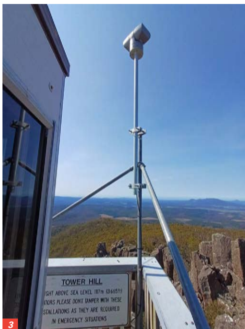
1 & 2/ The implementation of TIFCN has the potential to dramatically improve bushfire detection in Tasmania. 3/ Elevated cameras combine with AI detection tools and other sensors to spot and report fire activity quickly. Images: supplied
