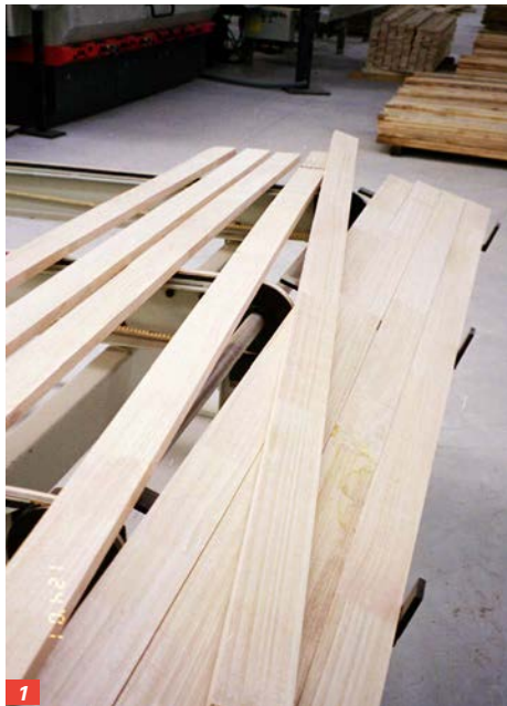
1/ Defect-docked E. globulus sawn wood prior to finger-jointing: Villapol S.A. 2/ Lamella after finger-jointing & ready for lamination: Villapol S.A.
