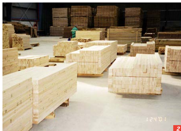
1 & 2/ The Villapol S.A. GLT products – three lamella window scantlings – for European markets. All photos: courtesy Evan Shield
