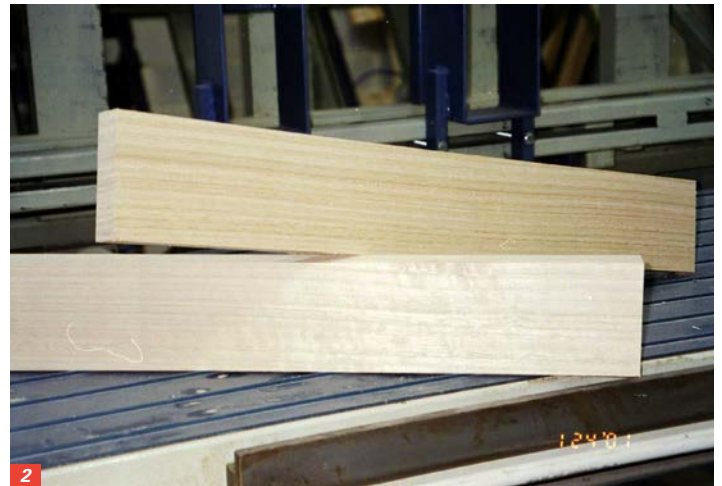
1/ Defect-docked E. globulus sawn wood prior to finger-jointing: Villapol S.A. 2/ Lamella after finger-jointing & ready for lamination: Villapol S.A.
