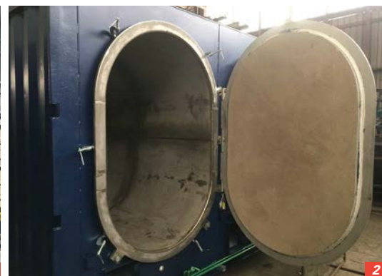
2/ Industrial pyrolysis combustion chamber. All images: Crusader Engineering
