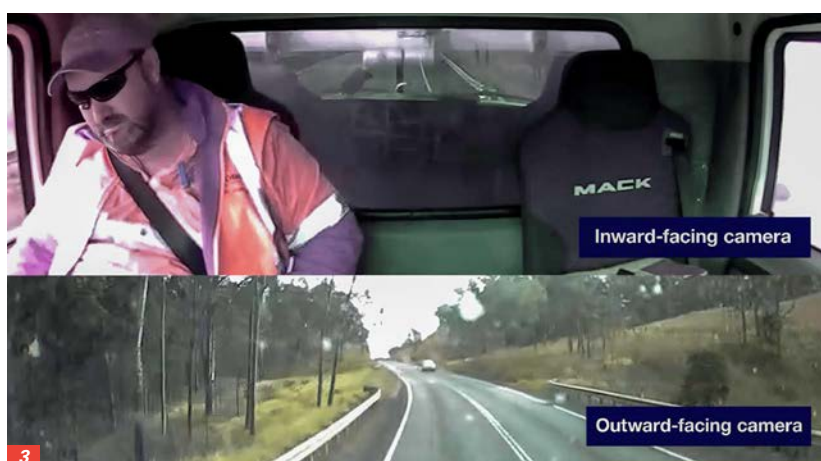
1/ Adbri Quarries have been running the AI cameras on 100 trucks, with positive results. 2/ The driver-facing camera is unobtrusive. Research shows that this type of monitoring system is much more effective than indirect systems. 3/ A driver nodding off for a moment in a microsleep will trigger the camera and sound an alarm. All photos: NTHA
