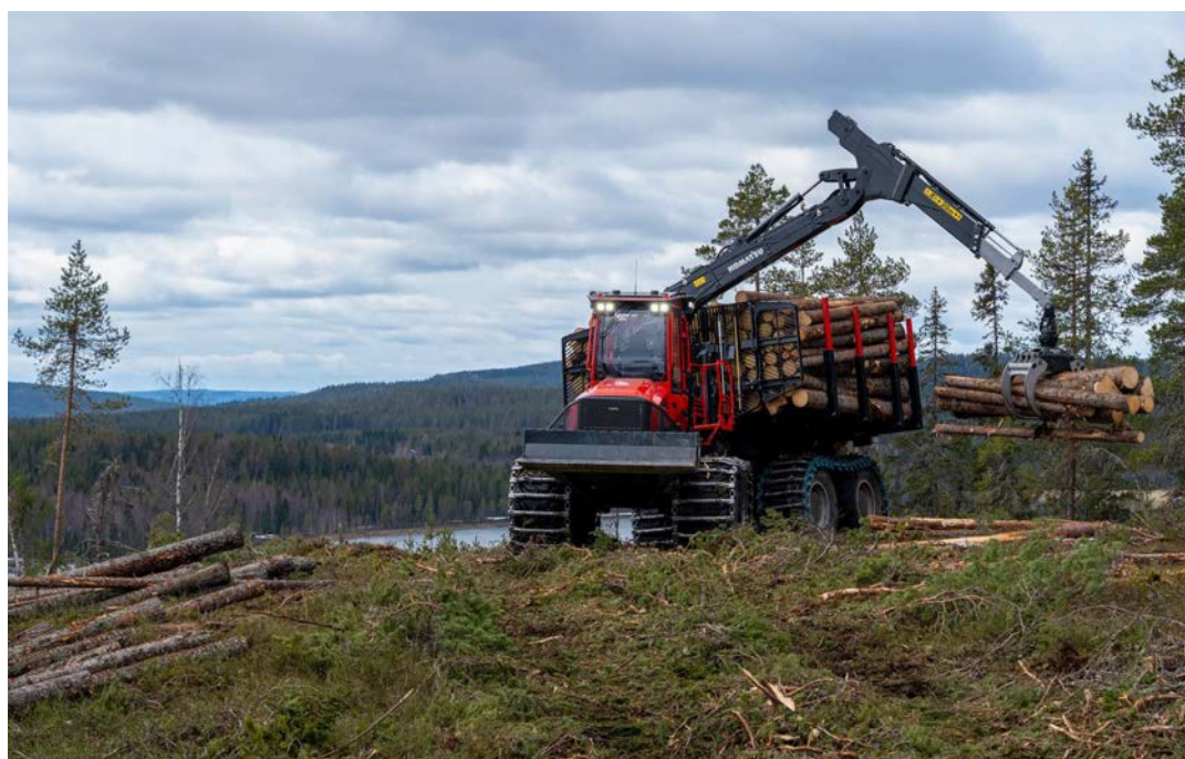
The new Komatsu 898 forwarder with 25 tonne load capacity. Image: courtesy Komatsu
