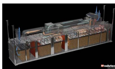
This diagram shows how the Closed Loop Drying system works. Photo: Accsys
