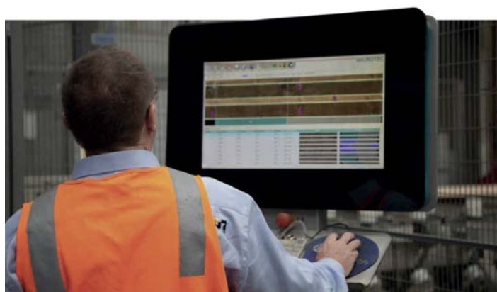
Snapshot of the MicroTec scanning machine's display screen, capturing the rapid scanning process of each timber board.
