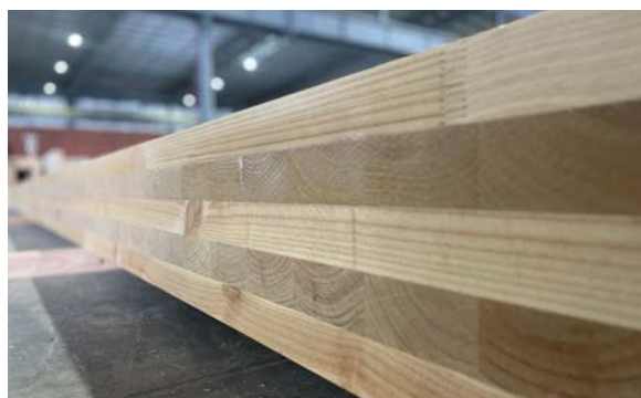
NeXTimber® Cross Laminated Timber (CLT) panels and Glue Laminated Timber (GLT) are produced with efficiency and precision at the facility.
