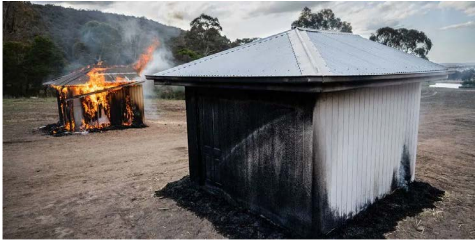
Shed with FSA Firecoat paint applied (right) versus shed without in a controlled real burn situation.
