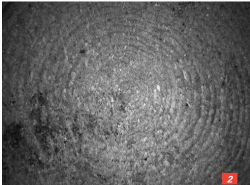
1/ A high-resolution camera mounted on the harvesting machine takes an image of each cut log surface and the context, which are stored together with a unique code.
