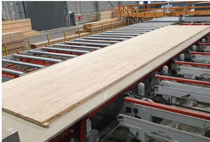
The first CLT panel pressed at the NeXTimber facility.
