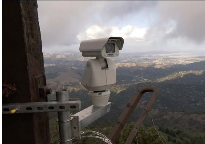
Similar camera-based fire detection systems have been installed on old fire watch towers in California.
