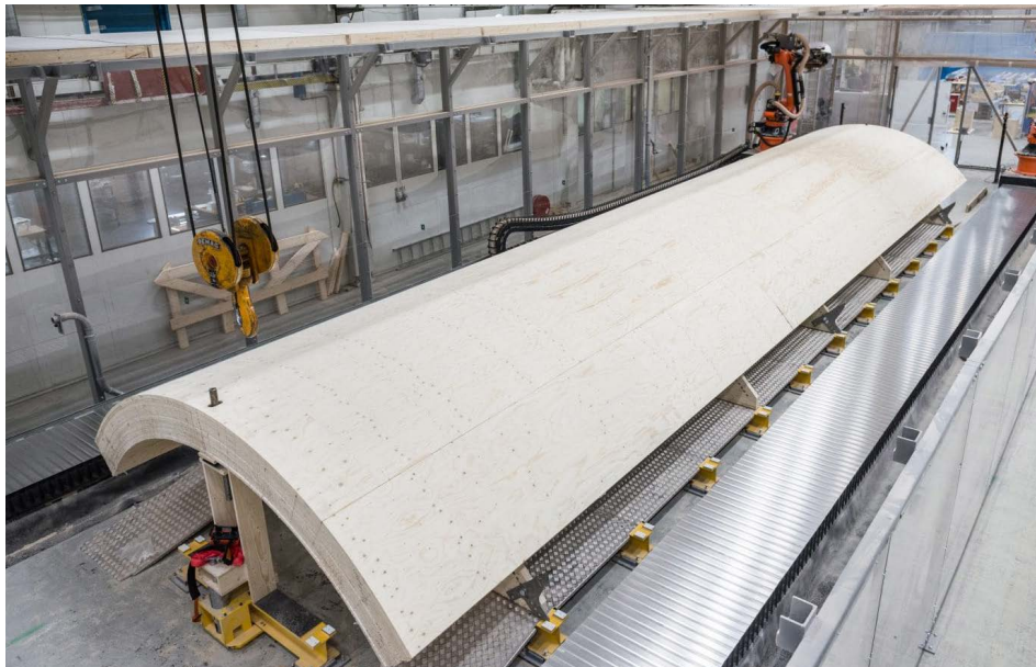
The companies have joined to produce laminated veneer lumber Modvion's wooden wind turbine towers.
