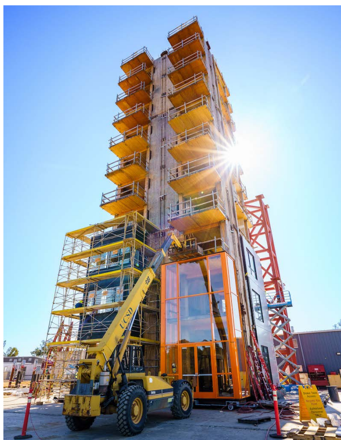
The Tallwood project will put to the test a 10-story, full-scale, cross-laminated timber building to assess seismic safety.
