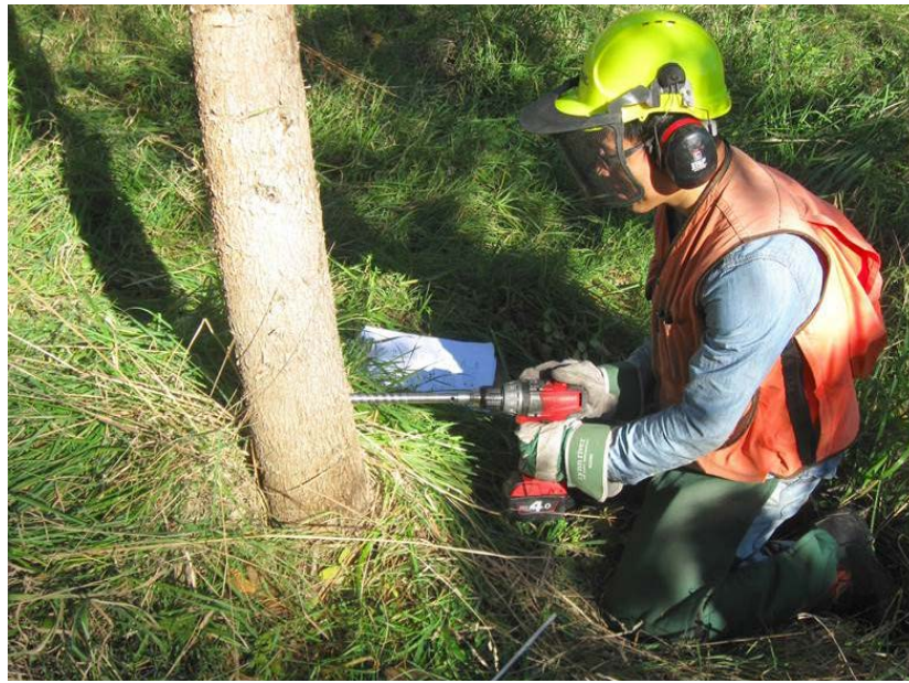
PhD student Yanjie Li uses a coring drill... part of research into predicting wood traits in durable eucalypts. Photo: NZDFI
