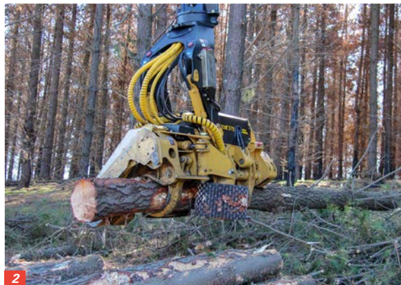
1/ High-performance... Tigercat 575 harvesting head impresses at in-field salvage trials in the Green Hills region of southern NSW where about 52,000 ha of radiata plantation was burned by the summer bushfires.
